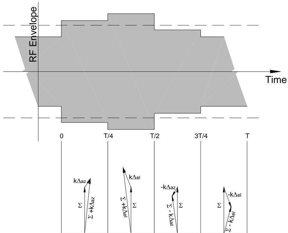
Figure 4. Coherent signal combination in the autotrack modulator. Phase errors in the  $\Delta az$  and  $\Delta el$  signals are exaggerated for clarity.
