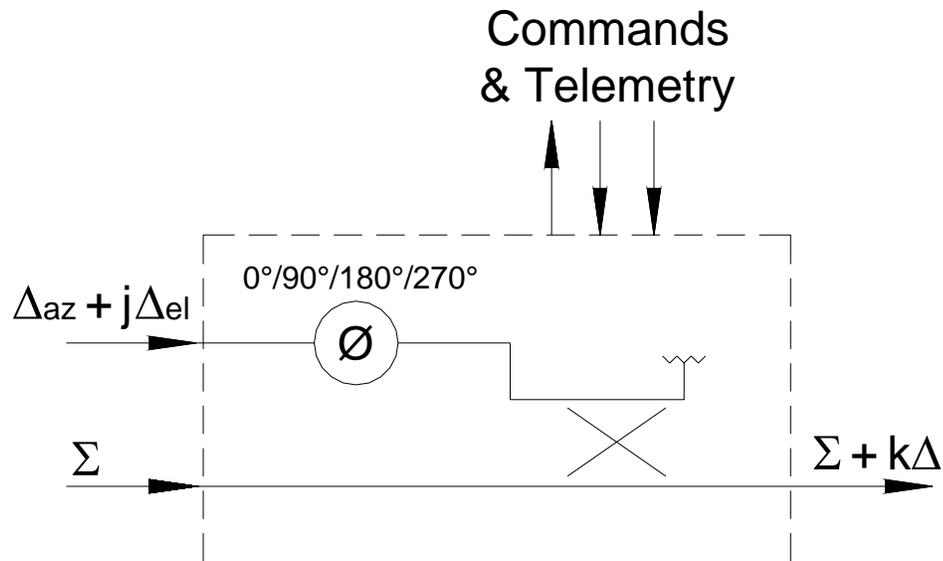
**Figure 11. In the phase shifter only autotrack modulator, the composite error signal is sequentially phase shifted in quadrature steps.**
