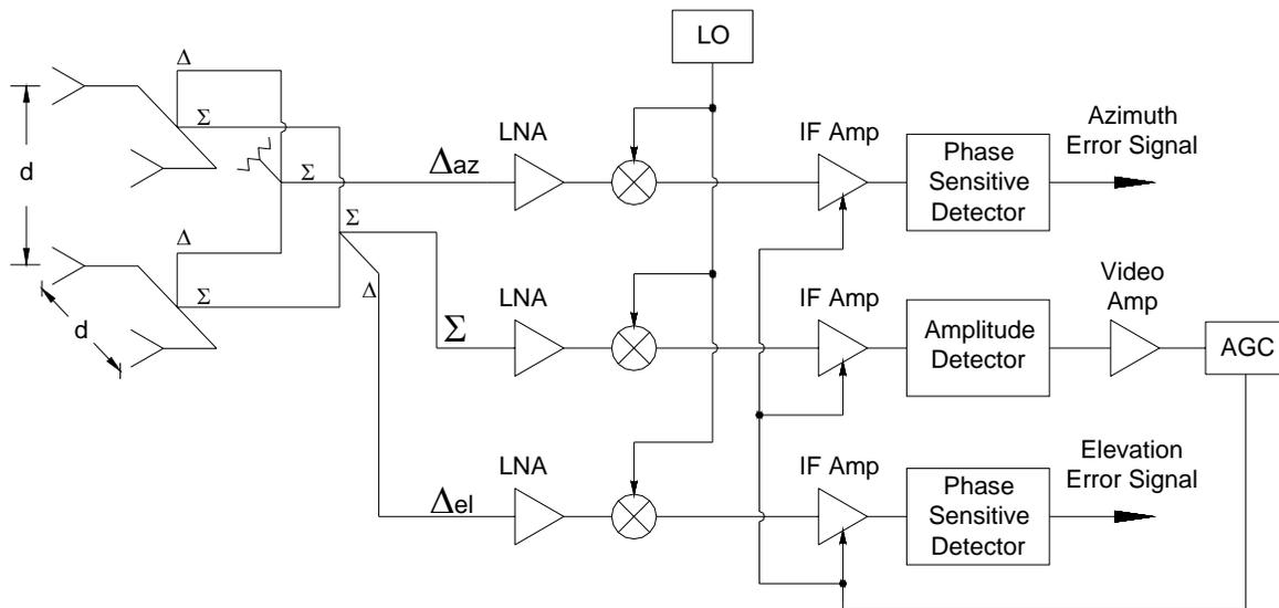
**Figure 1. A three-channel monopulse receiver system**
